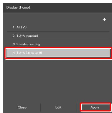
The remote control buttons are arranged according to the registered button layout.
