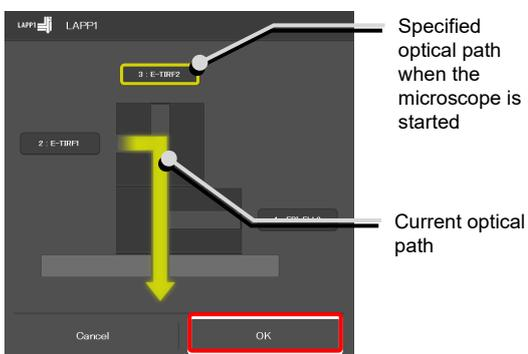
4. Repeat steps 1 to 3 for [LAPP2] when the upper and lower epi-illumination attachments are provided in a stage-up configuration.
