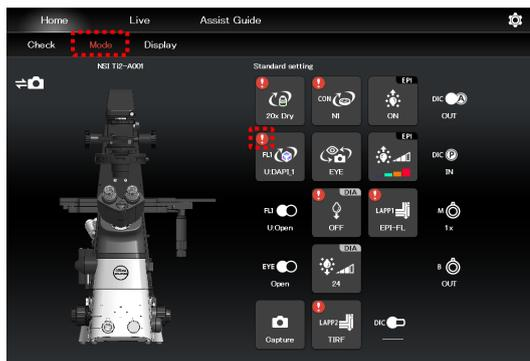
3. Tap the remote control button with the
