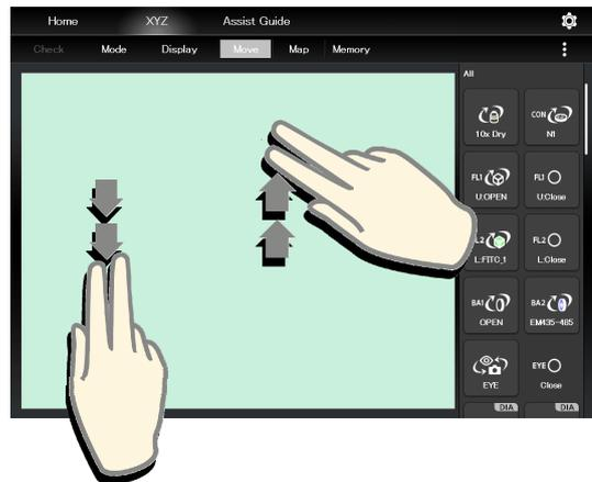
■ **Controlling the motorized stage (XY):**
