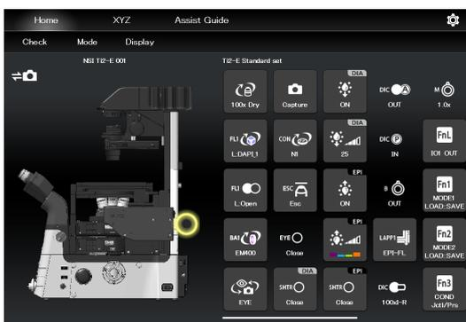
2. Tapping the [OFF] indication button turns the corresponding LED on. Tapping the [ON] indication button turns it off.
