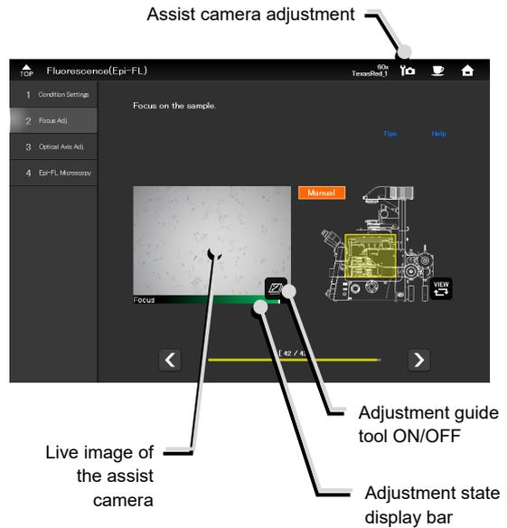
▼ **Optical axis adjustment (Example: Köhler illumination needing adjustment)**
