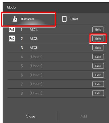
Select the [Tablet] tab and tap [Edit] of the desired mode number to display the screen of the mode in the tablet.
