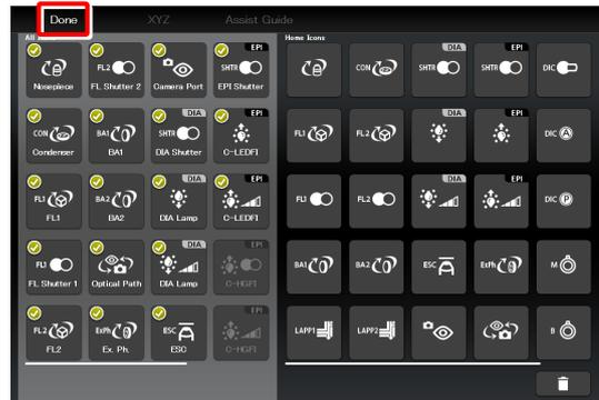
9. To save the customized button arrangement as a remote control button layout, specify a name in the [Name] field, and then tap [Save].
