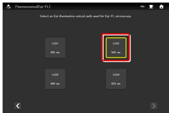
**When the D-LEDI is attached and Async mode is selected, select the wavelength of the light source used for epi-fl microscopy.**
