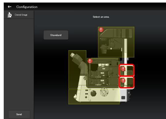
In a two-tier configuration, the upper and lower epi-illumination attachments are mounted in opposite directions. However, the application shows the two epi-illumination attachments in the same orientation.
