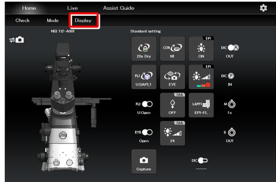
2. Select the name of the remote control button layout from the list, and then tap [Apply] to arrange the remote control buttons accordingly.
