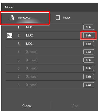
Select the [Tablet] tab and tap [Edit] of the desired mode number to display the screen of the mode in the tablet.
