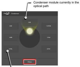
Long-tapping the name displays the detailed information about the condenser module
