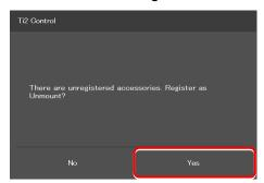
After the transmission, [Unmount] is displayed under the part without device information.
