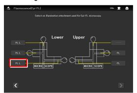
5. When the C-LEDFI is attached, select the wavelength of the light source used for epi-fl microscopy.
