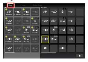
9. To save the customized button arrangement as a remote control button layout, specify a name in the [Name] field, and then tap [Save].
