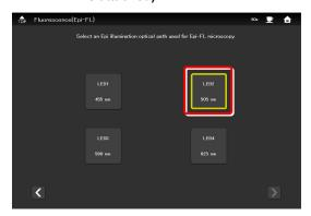
When the D-LEDI is attached and Async mode is selected, select the wavelength of the light source used for epi-fl microscopy.
